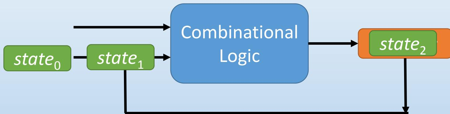
$$\begin{aligned}\# \text{ bitflips} &= \text{HD}(state_i, state_{i+1}) \\ &= \text{HW}(state_i \oplus state_{i+1})\end{aligned}$$
